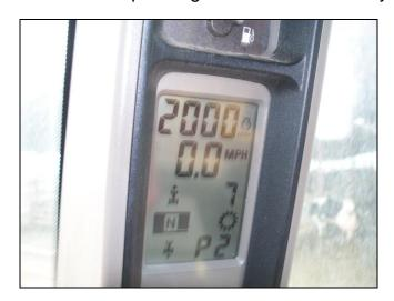
Once engine fluid levels have reached normal operating conditions the Carbon Balance study may begin. The above photograph shows that the engine RPM is locked in place at 2000 r.p.m. It should be noted that any deviation in r.p.m., temperature, either fluid or exhaust, would cause this unit to be eliminated from the evaluation due to mechanical inconsistencies.
