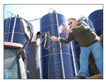
The above photograph shows one method in which exhaust pressure can be monitored during the Carbon Balance test procedure. In this case, exhaust pressure is ascertained through the use of a Magnahelic gauge. This type of stringent regime further documents the inherent accuracy of the Carbon Balance test.
