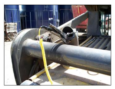
Once the exhaust temperature has stabilized, the test unit has reached its peak operating temperature. Exhaust temperature is critical to the completion of a successful evaluation, since temperature changes identify changes in load and RPM. As previously discussed, RPM and load must remain constant during the Carbon Balance study.
