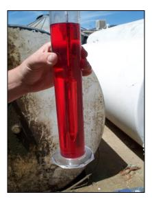
Fuel density and temperature tests are performed for both the baseline and treated segments of the evaluation to determine the energy content of the fuel. A .800 to .910 Precision Hydrometer, columnar flask and Raytek Minitemp are utilized to determine the fuel density for each prescribed segment of the evaluation.
