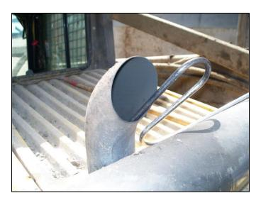
While the emission-sampling probe is in place, and data is being collected, exhaust temperature and pressure are monitored throughout the entirety of the Carbon Balance procedure. This photograph shows the typical location of the exhaust emissions sampling probe.
